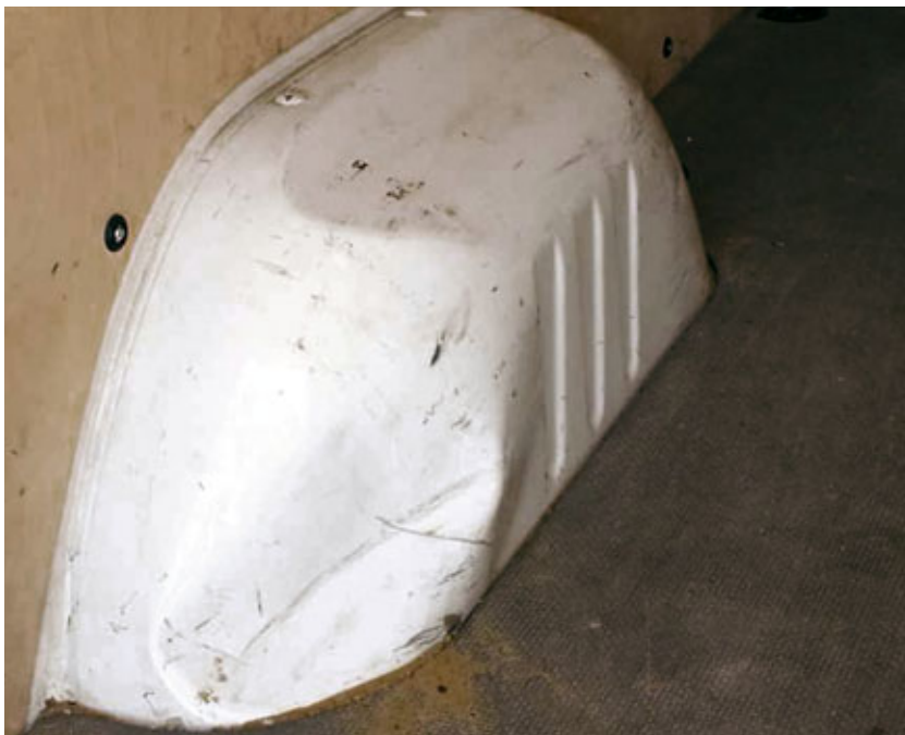
Deformation > 100 cm 2 am Radkasten
