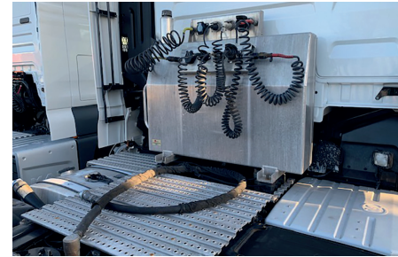
Auxiliary equipment: no distortion and pipework must be present and working.
