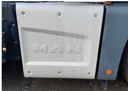
Exhaust heat shield: Discolouration acceptable - no distortion.
