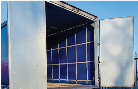
Tail lift rear opening: If applicable, removal of paint in loading area due to fair wear and tear.
