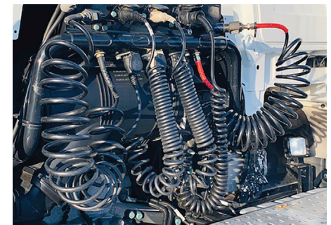
Couplings: Auxiliary equipment stowed correctly and present.
