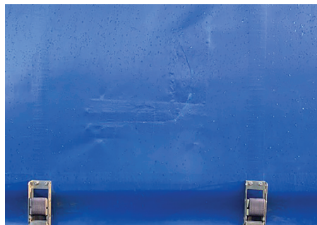
Curtain: Neat external curtain repairs.
