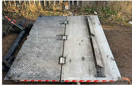
Tail lift: If applicable - Paint deterioration and surface rust on tail lift and fully operational.
