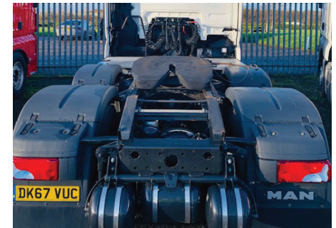
Rear view: If supplied as original equipment, lead up ramps, air lines, electrical leads should be present.
