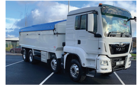
Dust sheets must be free from rips and in full working order.
