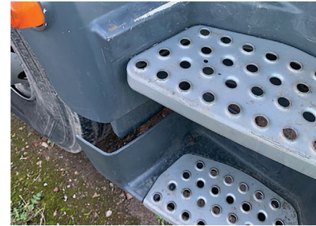
Paint wear steps: Paint surface worn but no distortion.
