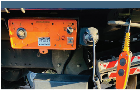
Tail lift operation 2: If applicable - Tail lift controls free from damage and fully operational.
