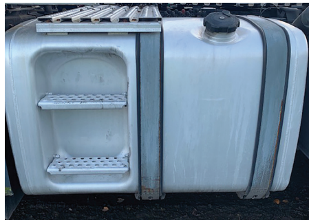
Fuel Tank Cap: Discolouration, and no distortion, MAN approved fuel and add blue cap.
